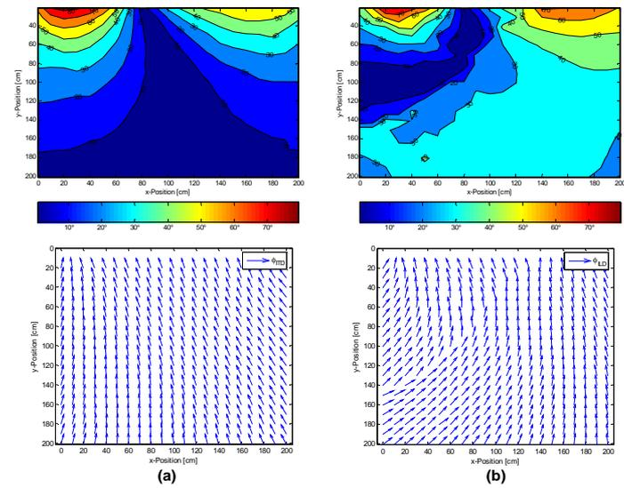
**Figure 6:** “Quality maps” (top) and “vector maps” (bottom) for time stereo ( $\Delta t = 0.14$  ms) with signal adjustment; **(a)** based on ITD cues; **(b)** based on ILD cues
