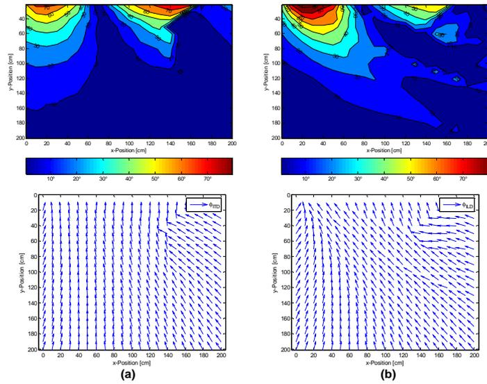
**Figure 5:** “Quality maps” (top) and “vector maps” (bottom) for “intensity” stereo ( $\Delta L = 6$  dB) with signal adjustment; **(a)** based on ITD cues; **(b)** based on ILD cues
