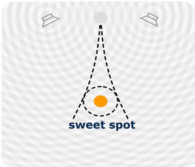
Figure 1: Schematic figure of the “sweet spot”
