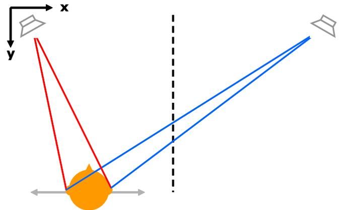
Figure 2: Asymmetric signal paths between loudspeakers and ears for an eccentric listening position
