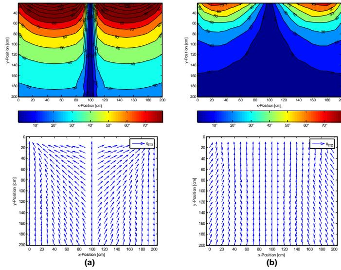
**Figure 4:** “Quality maps” (top) and “vector maps” (bottom) for a simulated center phantom source based on ITD cues; **(a)** without signal adjustment; **(b)** with signal adjustment
