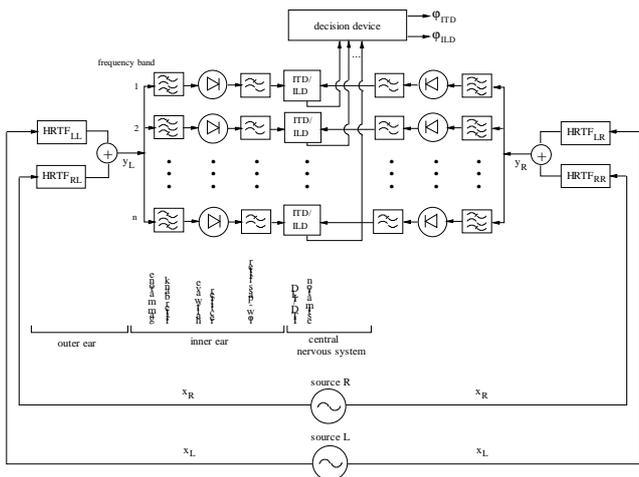
**Figure 3:** Adapted binaural model for phantom source localization in a stereophonic setup (after Braasch [4, 5])
